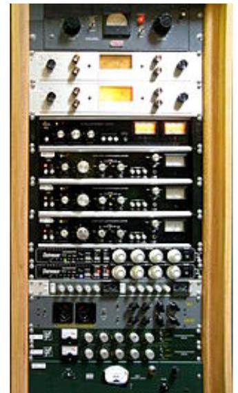
A rack of audio compressors in a recording studio. From top to bottom: Retro Instruments/Gates STA level; Spectra Sonic; Dbx 162; Dbx 165; Empirical Labs Distressor; Smart Research C2; Chandler Limited TG1; Daking FET (91579); and Altec 436c.
