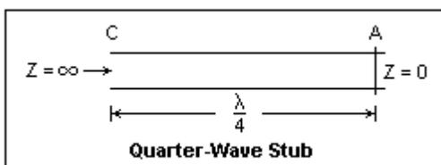
A quarter-wave line shorted at one end, as shown in the figure, is called a *quarter-wave stub*, and presents a very large impedance at its open end. Such stubs can be used to support a transmission line. Although there will be a DC path to ground, signal frequencies will be isolated. They will also act as pretty good bandpass filters, too, since only the signal current will not be shorted out.
