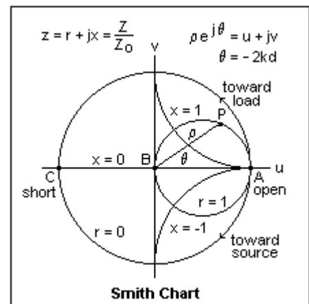
The normalized reactance,  $x$ , is also constant on circles which pass through A and have their centres on the  $v$ -axis. These circles are easily found to be  $(u - 1)^2 + (v - 2/x)^2 = (2/x)^2$ . The parts of the circles for  $x = +1$  and  $x = -1$  are shown. Positive, or inductive, reactance is above the  $u$ -axis, while negative, or capacitive, is below. The  $u$ -axis corresponds to  $x = 0$ , or a  $z$  that is purely resistive.
