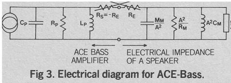
Fig 3. Electrical diagram for ACE-Bass.
