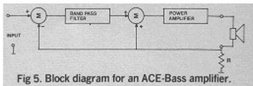
Fig 5. Block diagram for an ACE-Bass amplifier.
