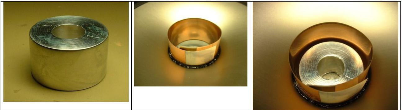
There are some pictures of the measurement system without gluing them in place. First picture is a closeup view of the inner cylinder made of aluminium, second is the outer cylinder, third shows how they will approximately be installed (just thrown in at that stage).
