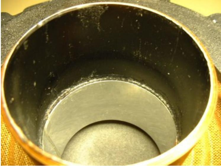
Voice coil former with outer cylinder of the measurement capacitor attached. This version is made from aluminium sheet.
