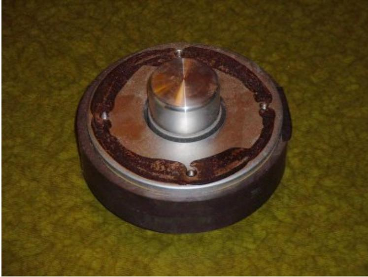
Magnet system. The aluminium cylinder on top of the polepiece is original one that will be replaced with similar "sandwiched" one that is presented in SEAS L18RNX-prototype.
