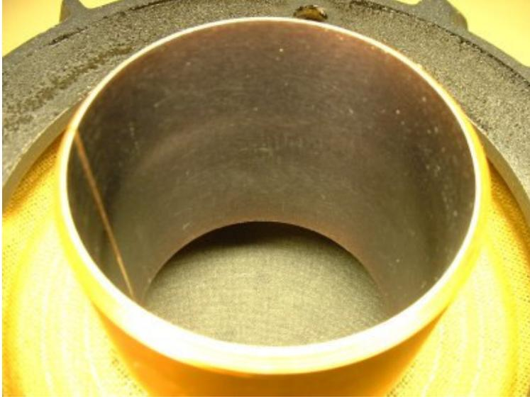
Voice coil former before attachment of the outercylinder of the measurement capacitor.
