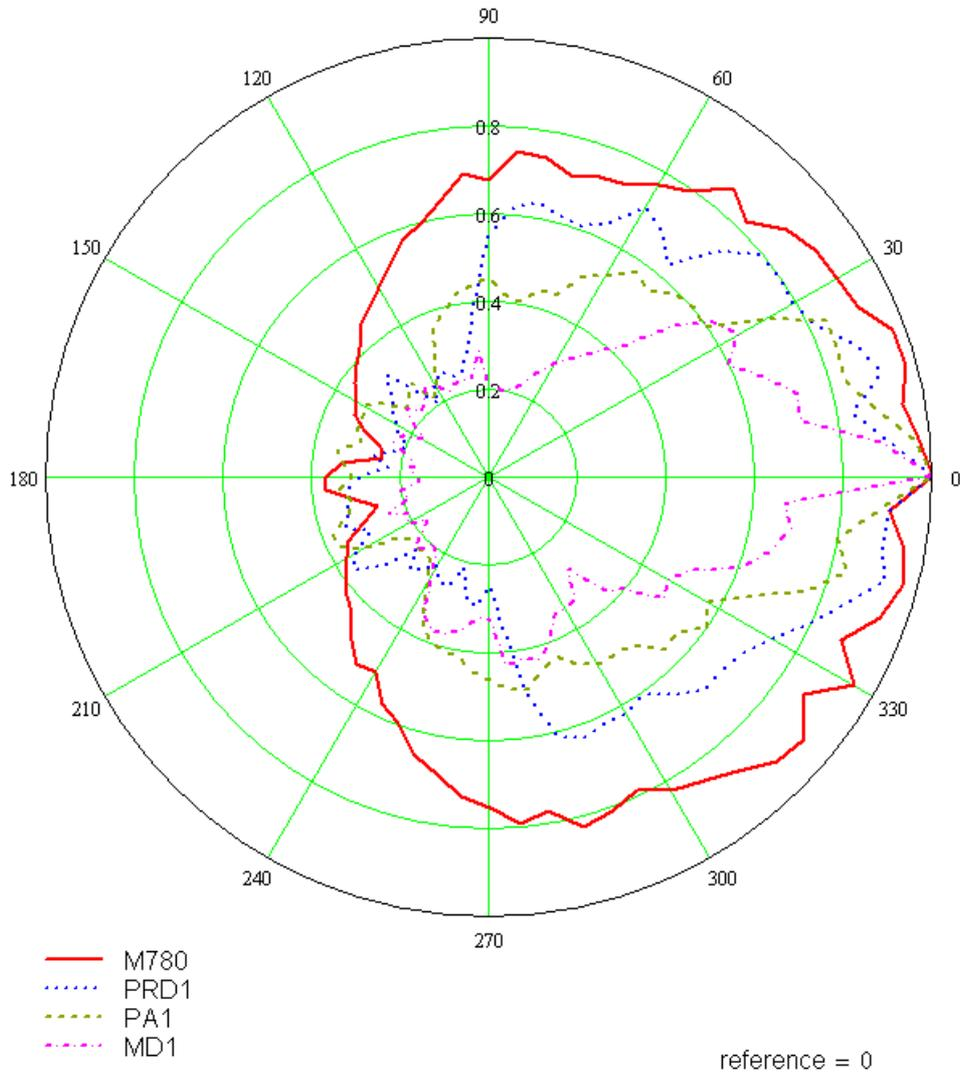
**Figure 1. Correlation directivity plots for four loudspeakers, using 0° reference.**
