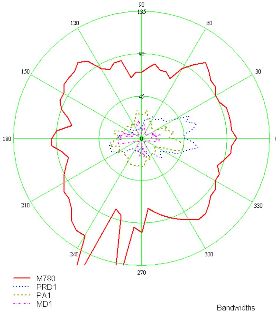
Figure 3. Spatial bandwidth vs. reference angle of loudspeakers by method 2
