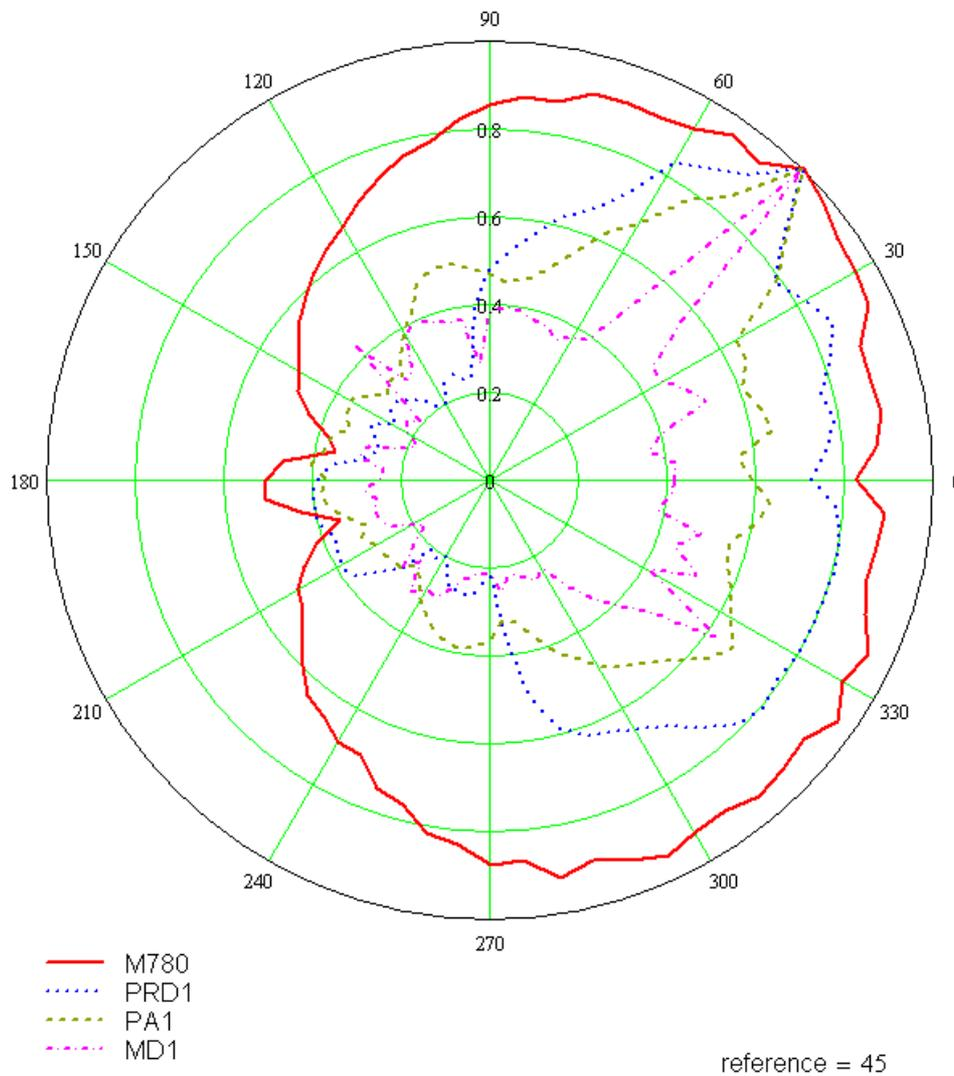
Figure 2. Correlation directivity plots for four loudspeakers, using 45° reference.
