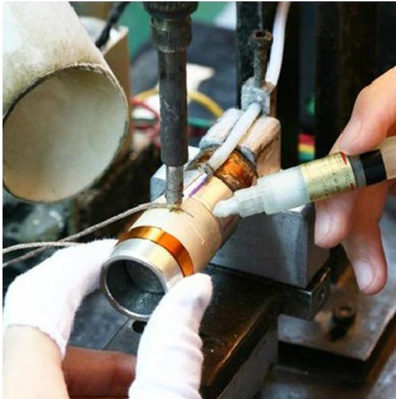
Photo 2: Voice coil winding and installing the collar (Source: Po Yun Enterprise Corp.)
