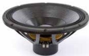
The system is made by two neodymium 18” or 21” subwoofers. The 5.3” diameter voice coil has been designed using the ISV inside-outside technology, enabling the transducer to handle up to 3600W program power with minimum power compression.
