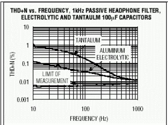
Figure 8. THD+N vs. frequency for large-valued, 100 $\mu$ F capacitors driving a 16 $\Omega$  load. Both types (tantalum and aluminum electrolytic) contribute heavily to THD at the nominal -3dB point of 100Hz. No such output-coupling capacitors are required with Maxim's DirectDrive headphone amplifiers.
