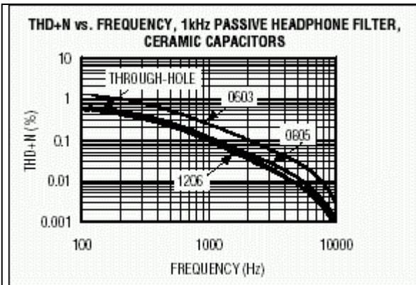
Figure 4. Comparison of THD+N vs. frequency for various ceramic capacitors in a 1kHz highpass passive filter.
