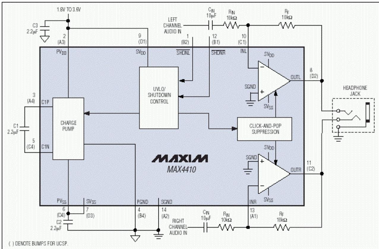
Figure 7. In this typical application circuit for the MAX4410 stereo headphone driver, setting  $C_{IN}$  to  $10\mu F$  restricts any voltage-coefficient effects to subaudible frequencies. Large-valued coupling capacitors at the output are not necessary.
