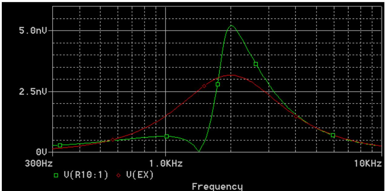
Note that the excursion is much reduced in the 800 Hz to 1.8 kHz region. The slope of the elliptic below 500 Hz is around the same as a regular 2nd order xover. But by this point the excursion is so low this fact doesn't matter.
