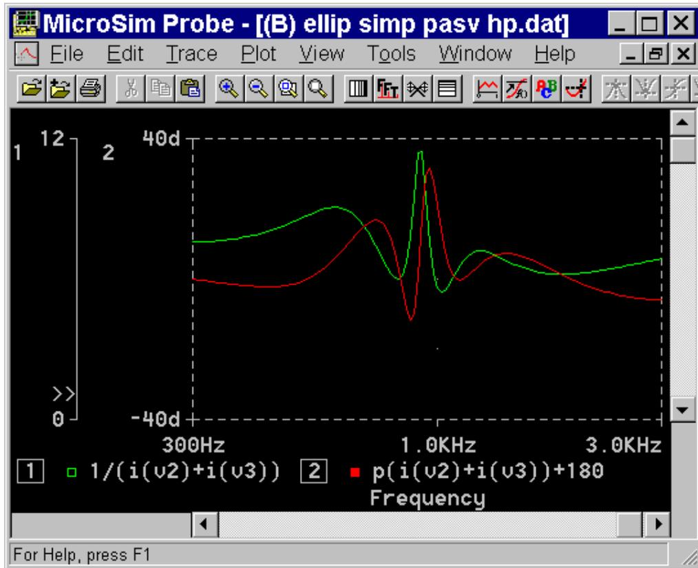
Green is impedance, red is phase. Impedance dips to 5.5 ohms, and phase is + 30 degrees max. Not too bad, but with 4 ohm drivers this drops to 2.7 ohms - beware. And, the impedance if the xover is biamped is not as benign.
