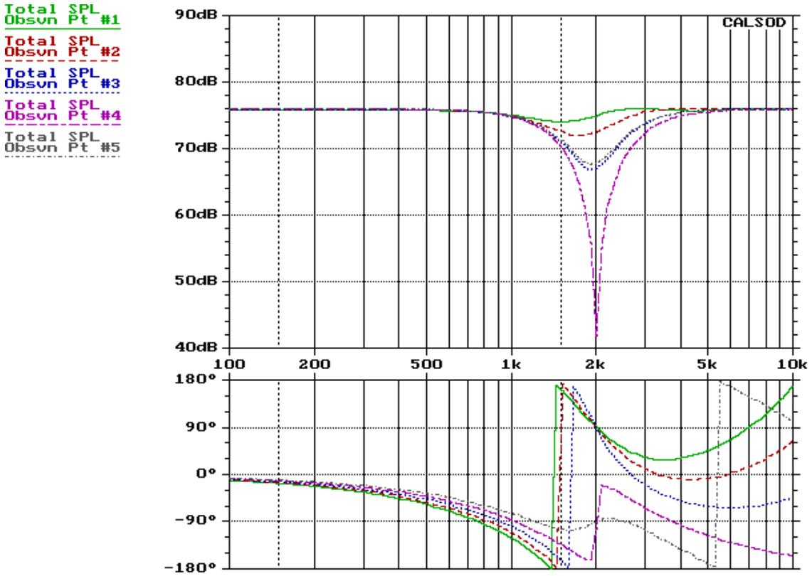
Note how superior the off-axis performance of the elliptic xover is compared to a 4th order L-R, for the cost of an extra capacitor!
