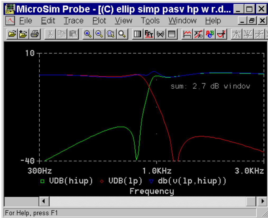
The effect was minimal. The ripple in the summation enlarged to 2.7dB, and the slope on the tweeter increased. Interference region is about the same
