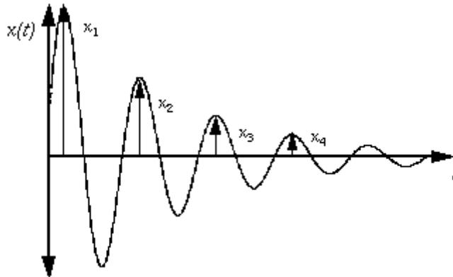
**Figure 2.1** Impulse response of a simple oscillator
