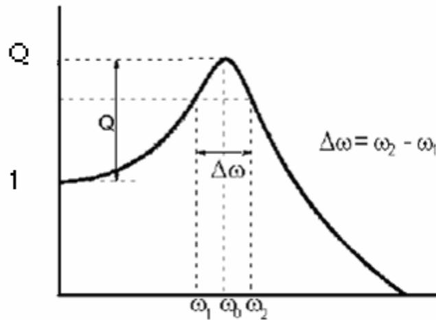
**Figure 2.2** Bandwidth method of damping measurement in a single-degree-of-freedom system.
