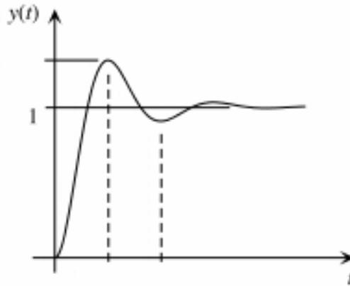
**Figure 2.2.** A typical step response of a simple oscillator
