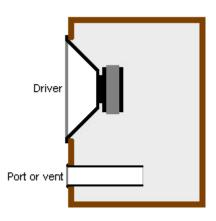
Bass reflex enclosure schematic (cross-section)
