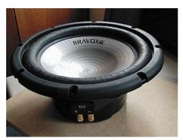
12-inch (30 cm) subwoofer driver (loudspeaker). A driver is commonly installed in an enclosure (often a wooden cabinet) to prevent the sound waves coming off the back to cancel out the sound waves being generated from the front of the subwoofer.
