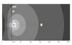
Cardioid dispersion pattern of two end-fire subwoofers placed one in front of the other. The signal feeding the enclosure nearest the listener is delayed by a few milliseconds.<sup>[66]</sup>
