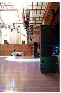
Each stack of speakers in this sound reinforcement setup consists of two EAW SB1000 slanted baffle subwoofers (each contains two 18-inch drivers) and two EAW KF850 full range cabinets for the mid and high frequencies.
