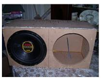
A homemade car audio subwoofer speaker box with a 15-inch Boss Audio subwoofer and an empty space for a second driver
