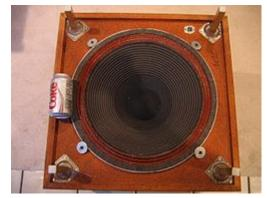
View of the underside of the downwardfiring Infinity Servo Statik 1, showing the size of the 18-inch (45 cm) custom-wound Cerwin Vega driver in relation to a can of Diet Coke, to show scale
