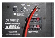
This picture of the rear panel of a Polk subwoofer cabinet shows a low-pass filter adjustment knob.
