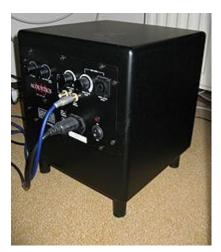
The rear panel of a down-firing, active subwoofer cabinet
